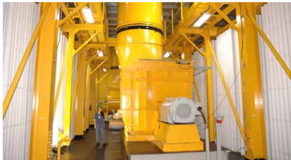
Sleeve filters for de-dusting, the largest filter of the kind in Latin America, with more than 17 thousand sleeves
